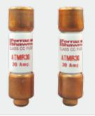
Amp-Trap<sup>\*</sup> ATMR fuses, in the Class CC family, are the smallest dimension 600VAC/DC fuses suitable for branch circuit protection. The ATMR is a popular choice for economical protection of control circuits and control circuit transformers where available short circuit currents exceed 10,000 amperes. ATMR's rejection dimensions prevent substitution by lesser rated fuses. These fast acting fuses give currentlimiting protection to general circuits.
